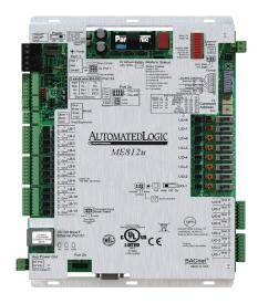
ME812u line controllers ave the speed, power, memory and I/O flexibility to handle the most demanding control applications in the industry. Capable of controlling
